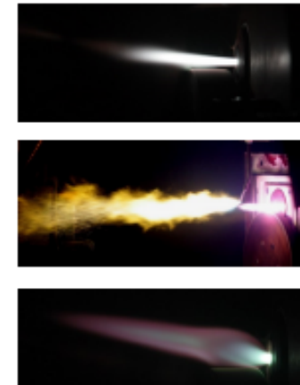
Plasma spraying torch WSP®H 2000 with hybrid stabilization:
